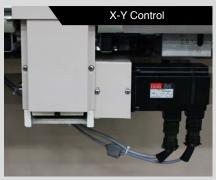
Control X Y position by sunstar servo motor implementing super fine control
