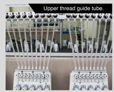
Stabilize the upper thread by upper thread guide tube (Supplied as standard components)
